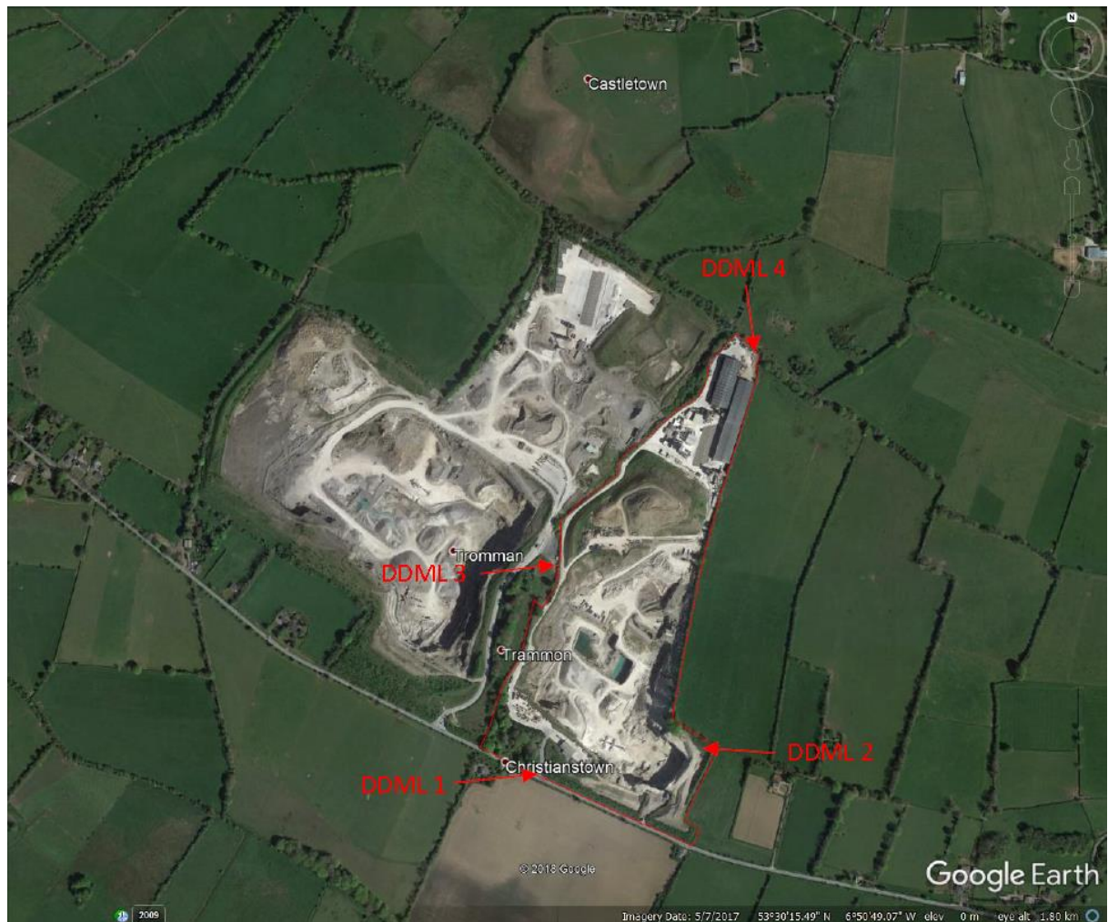
Figure 10.1: Dust deposition monitoring locations (DDML).
